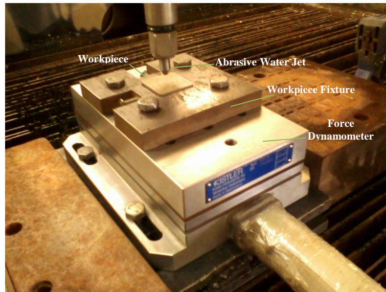
Fig. 3.4: Experimental setup photograph for pocket milling
